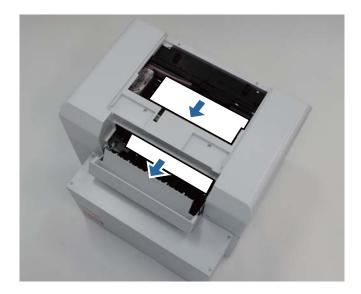
Move the Print head unit manually, and remove the paper from the rear.
